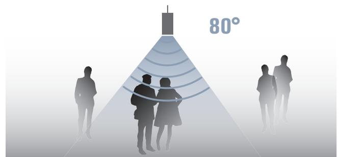
Minimum lateral sound radiation and a short distance allows focused acoustic irradiation to the visitors.
